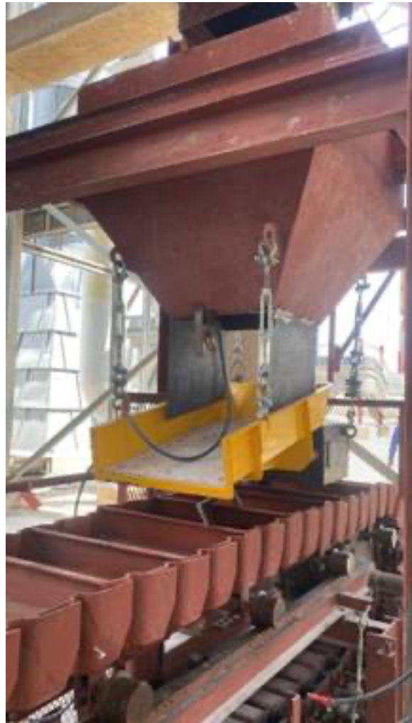
Figure 1: View of discharge and slide gates (left) and vibratory feeder above pan conveyor (right).
