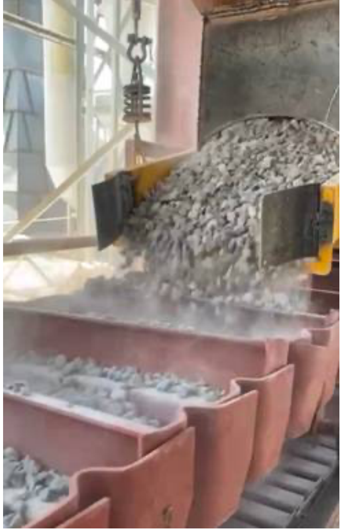
Figure 2: Skip with -90 to 60mm material at top of Kiln 1 (left); emptying limestone from Kiln1 (right).
