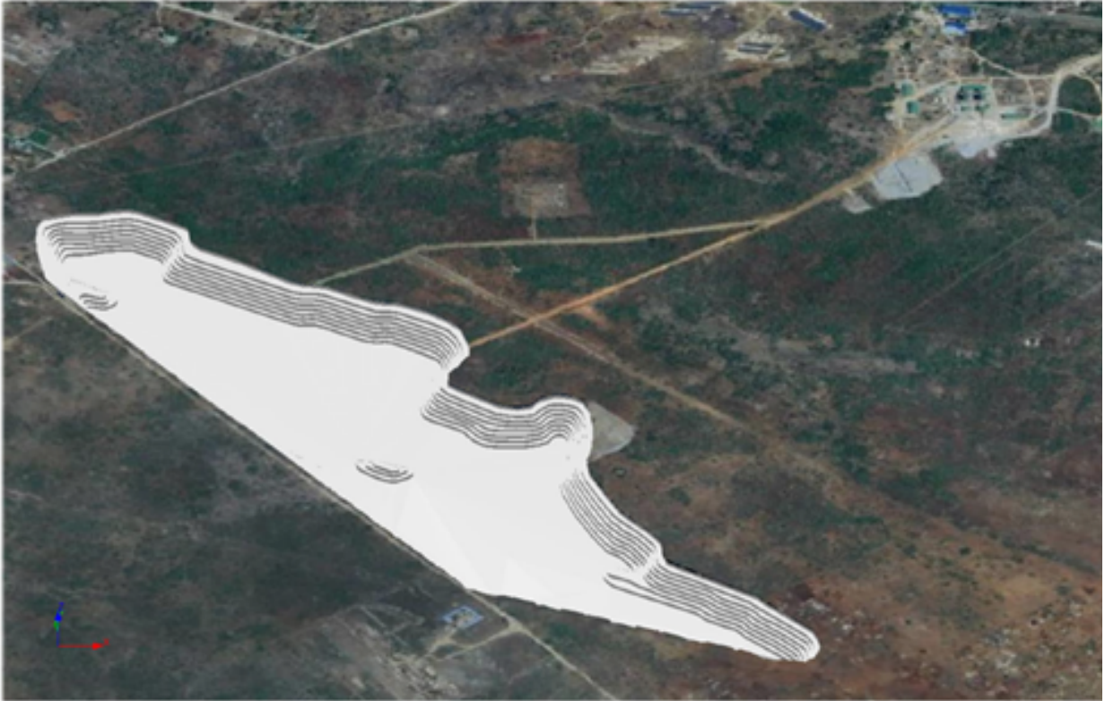
Figure 3: Representation of the pit shell; the lime plant can be seen in the upper right corner (Earthlab, November 2024).
