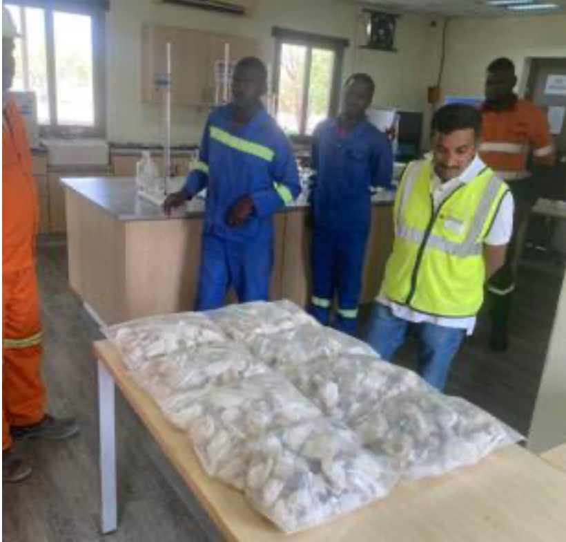
Figure 7: Burnt limestone from the pilot kiln awaiting further testwork to determine available quicklime (CaO).
