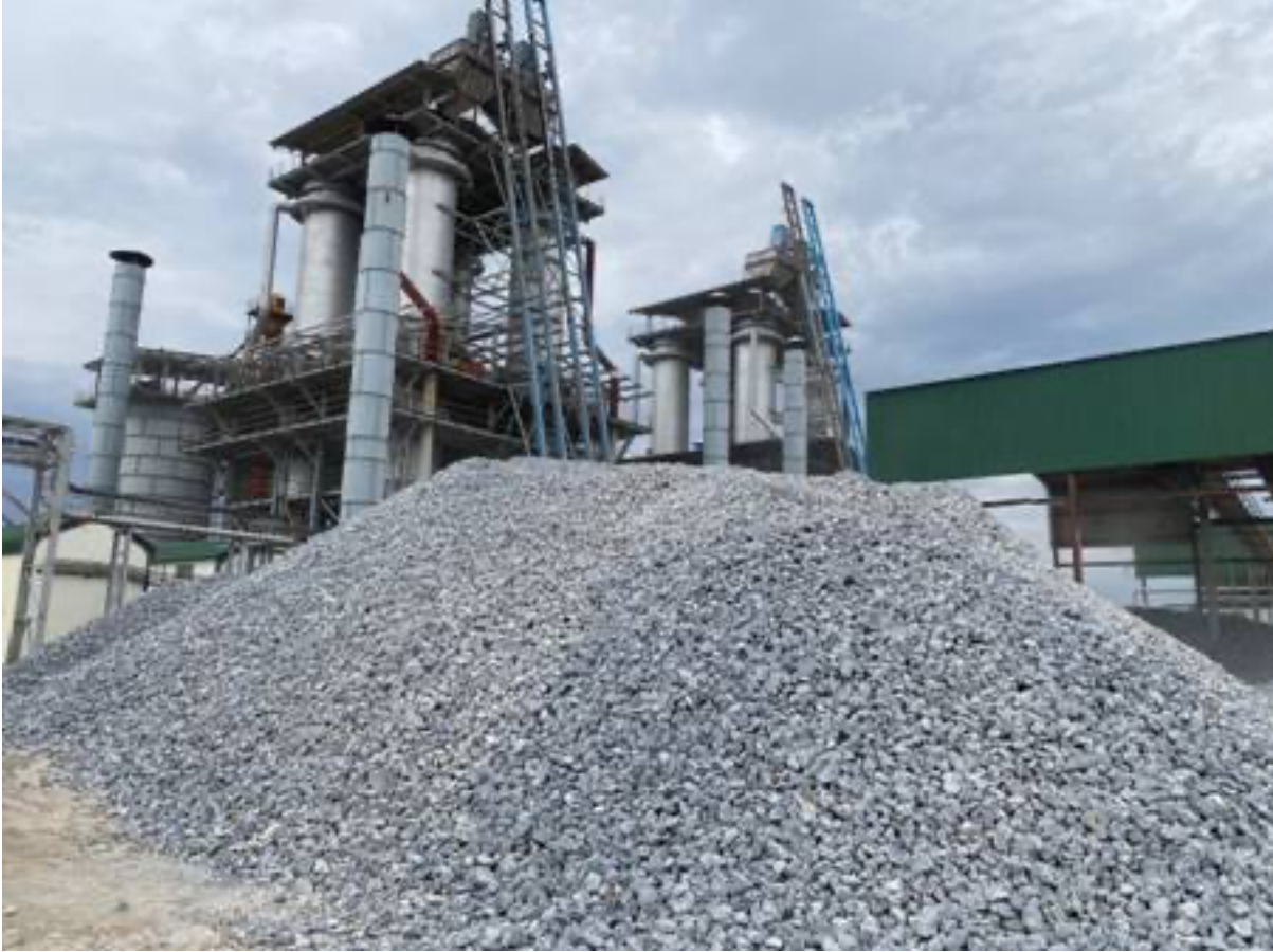
Figure 6: View of part of the kiln feed with lime plant in the background.
