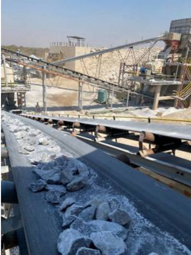
Figure 6: Belt feeding the -90mm to 60mm size fraction to the kiln feed pile.
